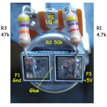
P1, P2 and P3 are the connection pads on the RM][ v3 PCB
